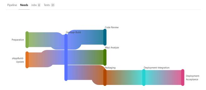
Depending on the availability of runners and dependencies relationships, the global execution of pipelines can be optimized when using this GitLab CI/CD capability.
